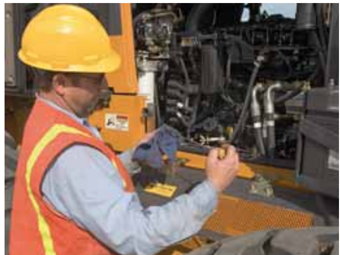
Drop-down side panels improve access to engine components and daily check points.
