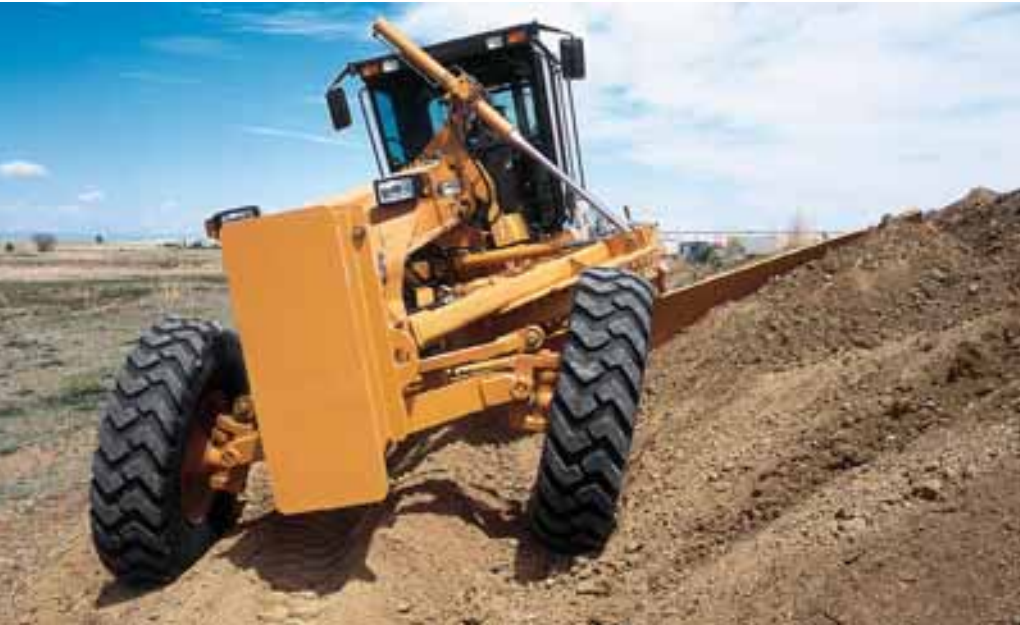
Front wheels lean for traction and moldboard control.
