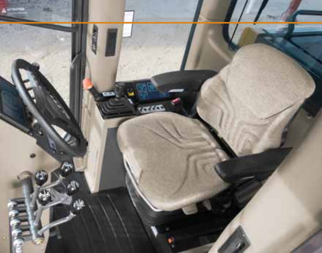
Low-effort control levers are positioned within easy reach and extended for operator comfort.
