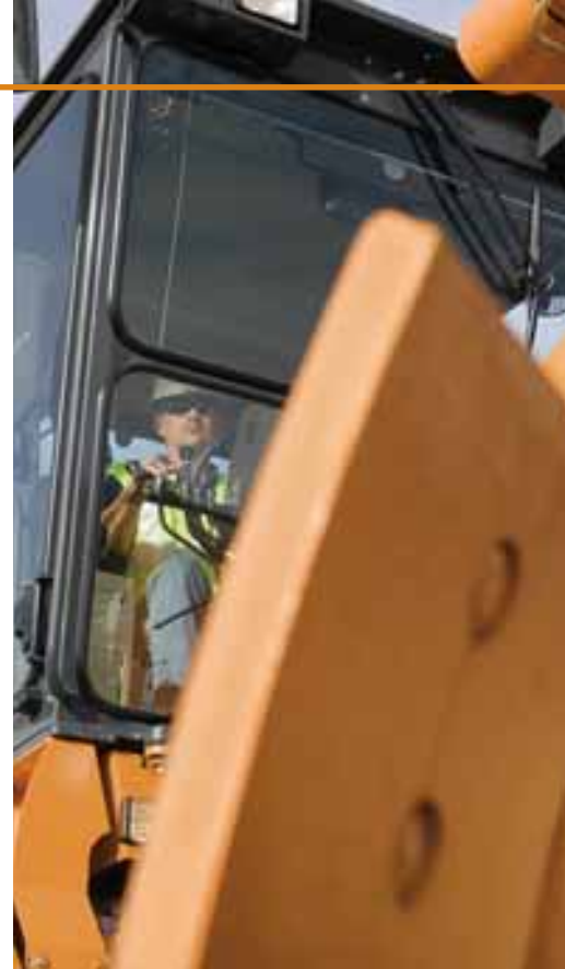
Floor-to-ceiling cab glass provides a clear view of the moldboard and superior all-around visibility.
