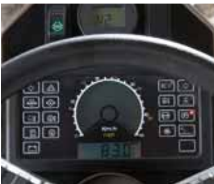
All important machine functions are monitored with dash-panel warning lights.
