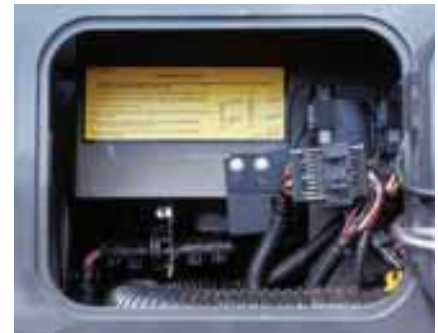
A convenient service door located on the side of the cab allows easy access to electrical connectors without removing interior cab panels.
