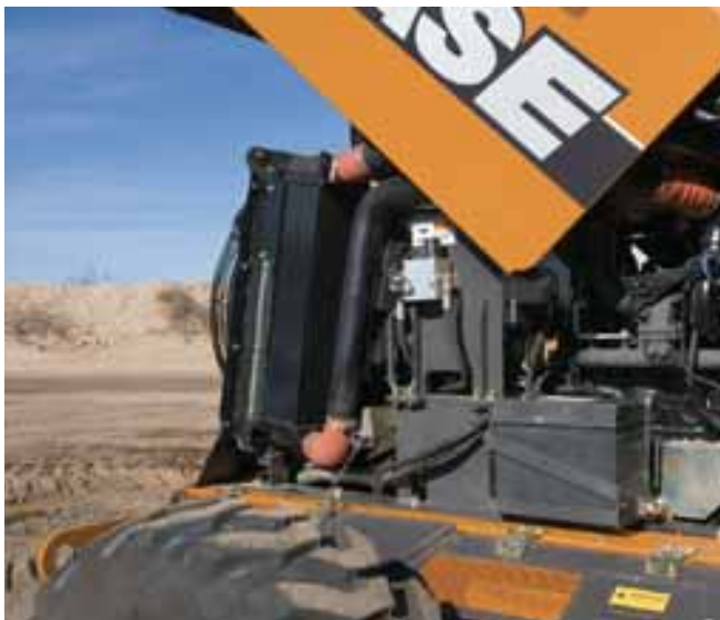
Drop-down side panels improve access to engine components and daily check points.
