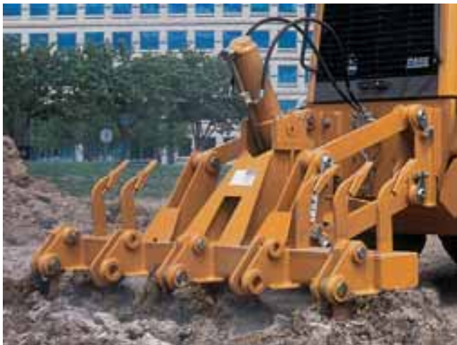
Rear ripper includes up to five teeth (three standard).
