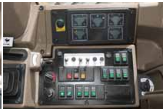
Analog gauges, attachment control, idle management, and diagnostic control are within easy reach.
