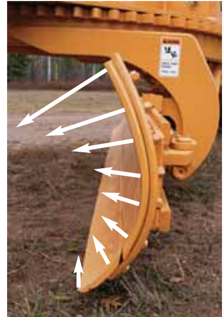
Multi-radius involute moldboard design cuts, mixes, and rolls material off the moldboard with decreased effort. The design increases the volume of dirt moved with less horsepower required and increased fuel economy. The boron-reinforced blade provides longer life when compared to the competition.
