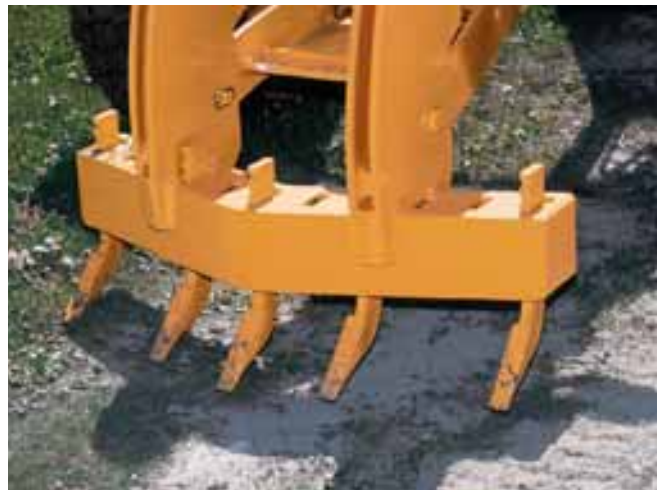
Front scarifier has up to 11 teeth (five standard).
