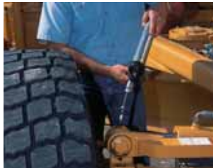
All grease zerks are easily accessed from ground level to speed daily service duties and increase productivity.
